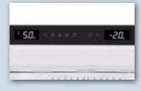
The electronic controller with digital temperature display allows accurate temperature setting to 1/10°C. The large display allows improved temperature visibility at a glance.
